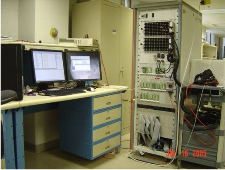
Fig. 2. body electronics hardware in the loop facility
